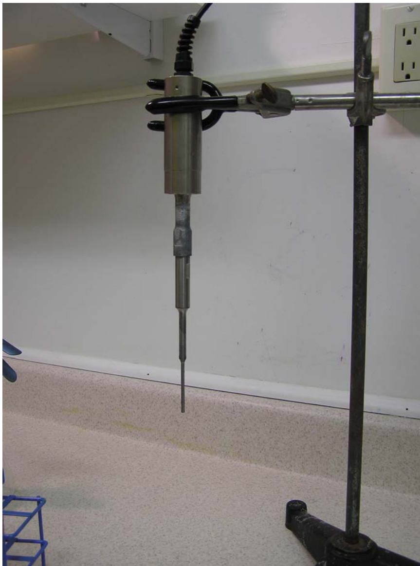
Typical Ultrasonic 'Sonicator' drive unit connects to an electronic control unit.
