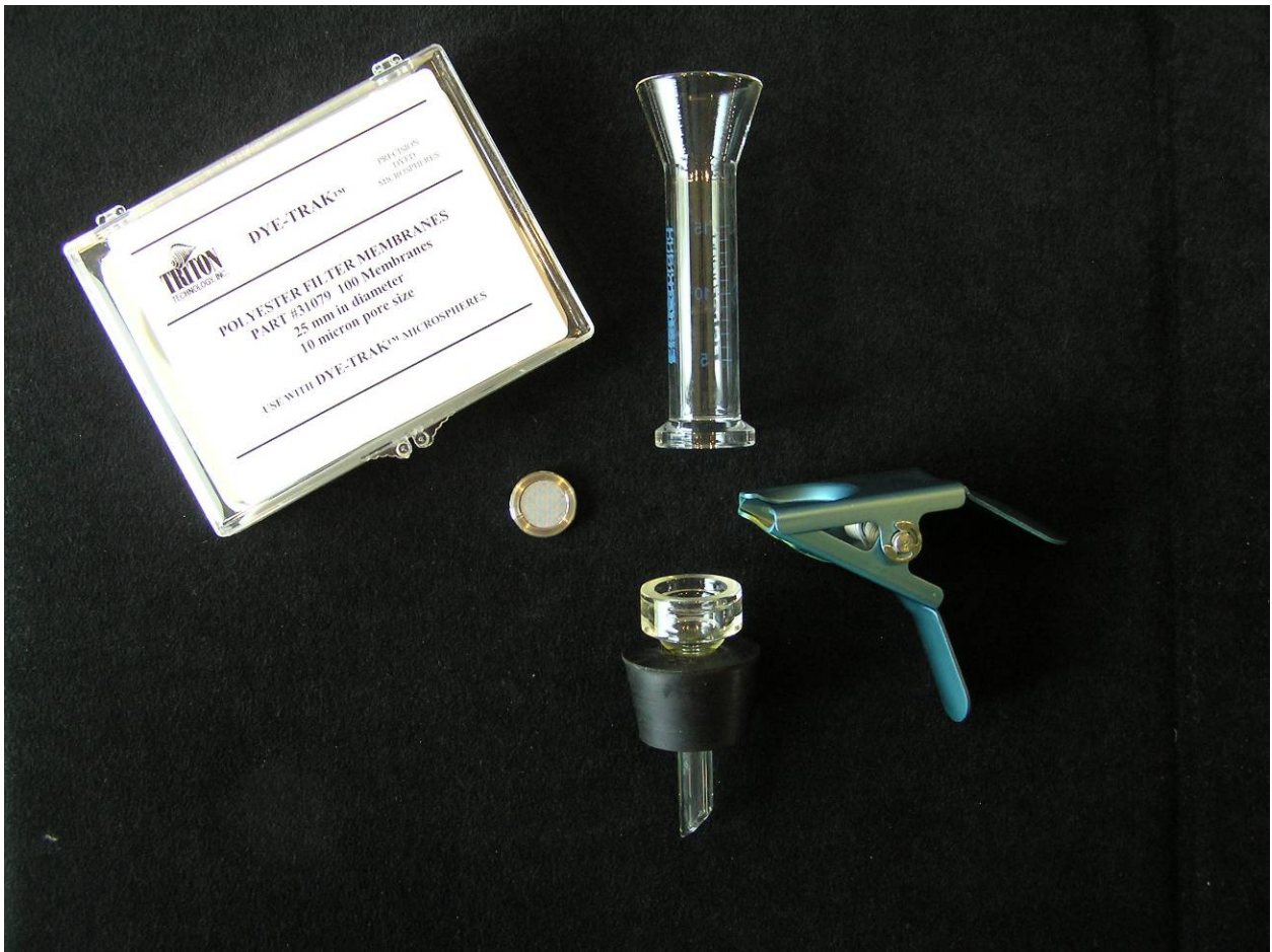
Typical vacuum filter apparatus for 25mm diameter filters
